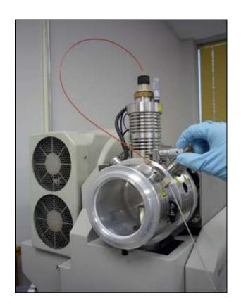
Mass Spectrometer Ion Source Housing
