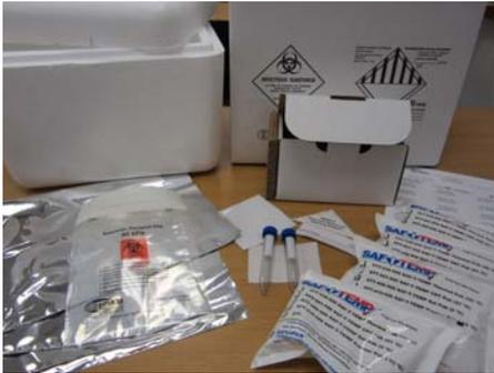
Figure 1. Example of materials needed to ship Category A infectious substances.
